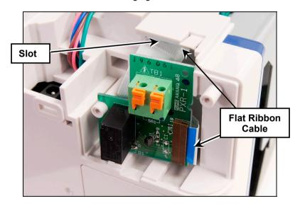
Insert the Time Signal PCB (PXR-1) into the cavity in the bottom of the PIX-200 as illustrated in the following figure – bottom view (the PCB assembly is notched so the assembly can only be inserted into the cavity in one direction). Please hold the edge of the PCB to avoid damaging the PCB.
