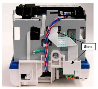
11. Insert the folded ribbon cable into the top center ribbon connector (see the wider cable in the following figure). Be careful not to damage the ribbon cable during insertion. When fully inserted, the cables' degree of insertion should be similar as indicated by the white arrows.
