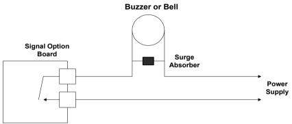
Figure - Time Signal Wiring Diagram
