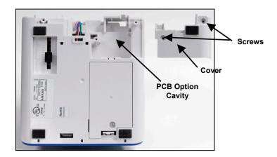
7. With the cover off, insert the Time Signal PCB ribbon cable through the slot as illustrated in the following figure - *bottom view*.
