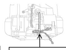
In order to feed the wires through the hole of the back plate, secure the wires using the cable tie as shown above. 7. Plug the power back in (disconnected in Step 5). Feed the AC power cable through one of the back plate holes, and the time signal wire through the other hole (see the following figure). Reattach the back plate, ensuring the tab is fully inserted. Refer to PIX-200 Operation Manual "Wall Mounting" if the PIX-200 is wall mounted.
