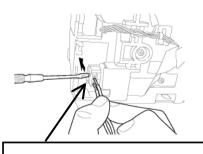
Press the orange protrusion of the terminal block downwards using a small flathead screwdriver when inserting the wires
