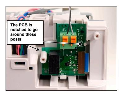
9. The PXR-1 PCB for the Time Signal Option will snap into place under a tab (see the following figure – *bottom view*). Use care to push the tab aside if necessary.
