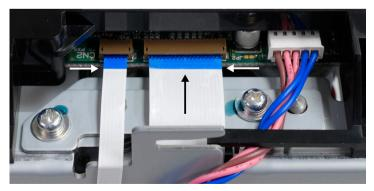
13. Be sure the flat ribbon cable also goes under the black plastic arm (see above figure). Place the option cover back on, and screw in the two (2) screws to tighten the cover down.
